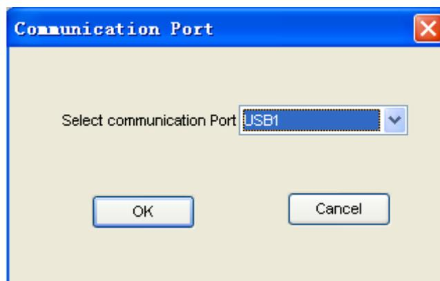
**Step 3.** Select the corresponding USB port (e.g.: USB1) for the PD78X, and click "OK" to enter the "Read" dialogue box as follows.
