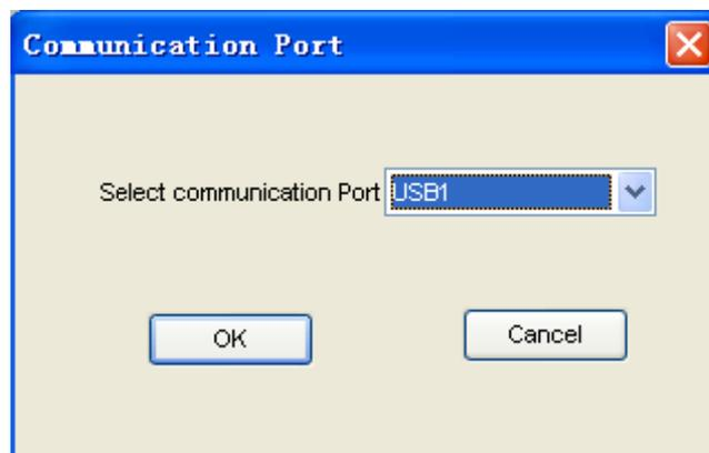
**Step 3.** Select the corresponding USB port (e.g.: USB1) for the RD98X, and click "OK" to enter the "Read" dialogue box as follows.
