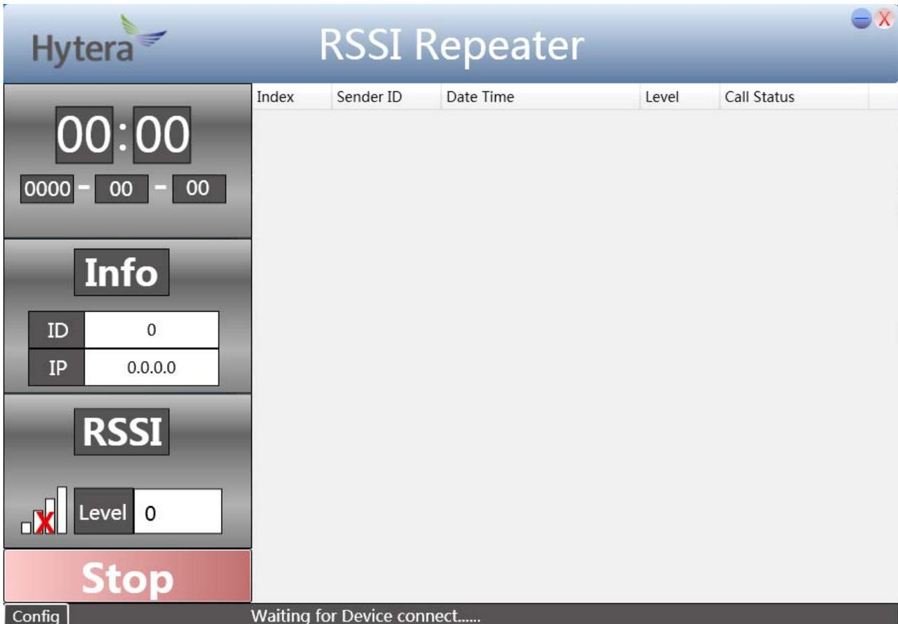
**Step 3.** The application will automatically connect the repeater about 2 minutes. After it is online, it will prompt "Device: XX is connected". "XX" indicates the repeater ID.
